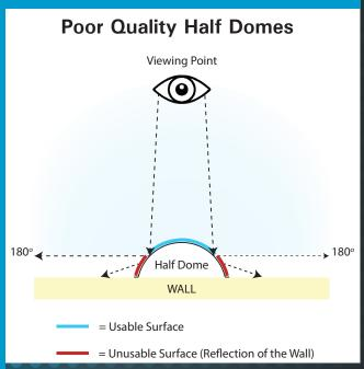
Other poorly made Half Dome mirrors are inferior because their curvature is too great. Their mirrors reflect "50% of unusable wall and ceiling area" resulting in the images being up to "50% smaller". The photo below shows the deep curve of these mirrors reflect a small image of the room and a large part of the wall.
