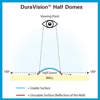
DuraVision™ Half Dome mirrors have a specifically designed curvature. This scientifically engineered curvature gives the "maximum usable reflective surface for a wideangle view" and more importantly, a "larger image size". The photo below shows the image of the corridor fills almost the entire mirror face.
